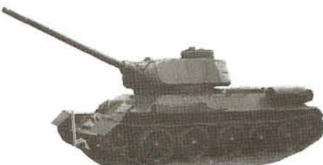
T34/85 — most heavily produced Soviet tank — over 19,000 made. This particular one was captured in the Korean War.
